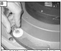
Install 4 Max. 15 watt bulbs into the sockets on top of the fan as shown.
